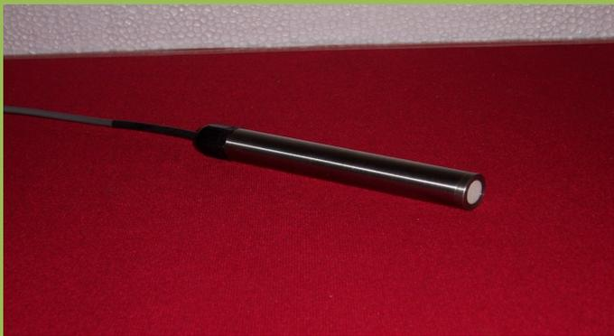
**Digital Water Level Monitoring System (Piezometer)**
