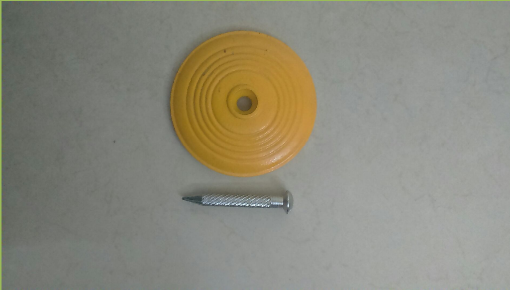
Pavement Settlement Points
